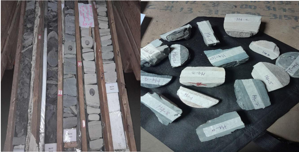
Figure: 3.1(a): Adigrat sand stone core sample Figure: 3.1(b) selected core samples
