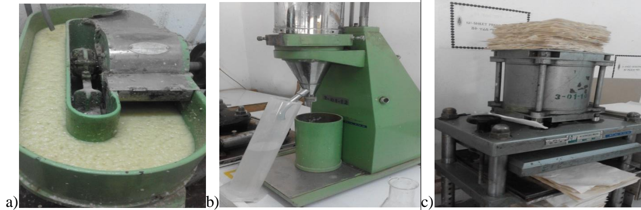
Figure A4: Beater machine (a), Freeness tester (b) and sheet molding (c)
