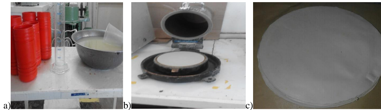
Figure A5: Prepared pulp slurry for sheet forming (a) Un-dried sheet (b) Dried paper sheet (c)
