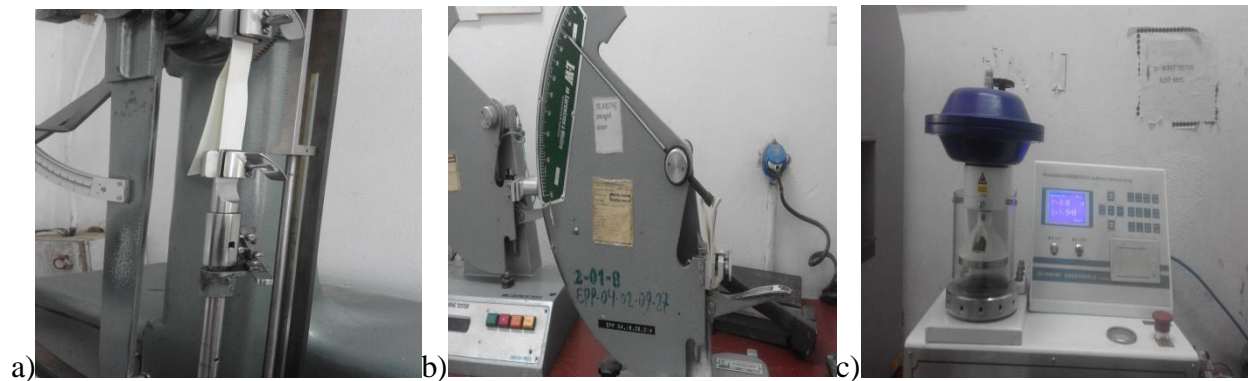
Figure A6: Tensile strength tester (a) Tear strength tester (b) and Burst strength tester (c)
