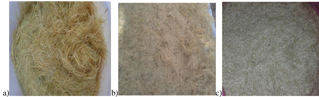
Figure A1: Raw material washing (a), Drying (b) and Size reduction (c)
