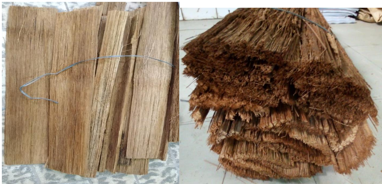
Figure 3-1 bamboo fiber partially extracted and thermally treated at 1600c for 3hr from African bamboo
