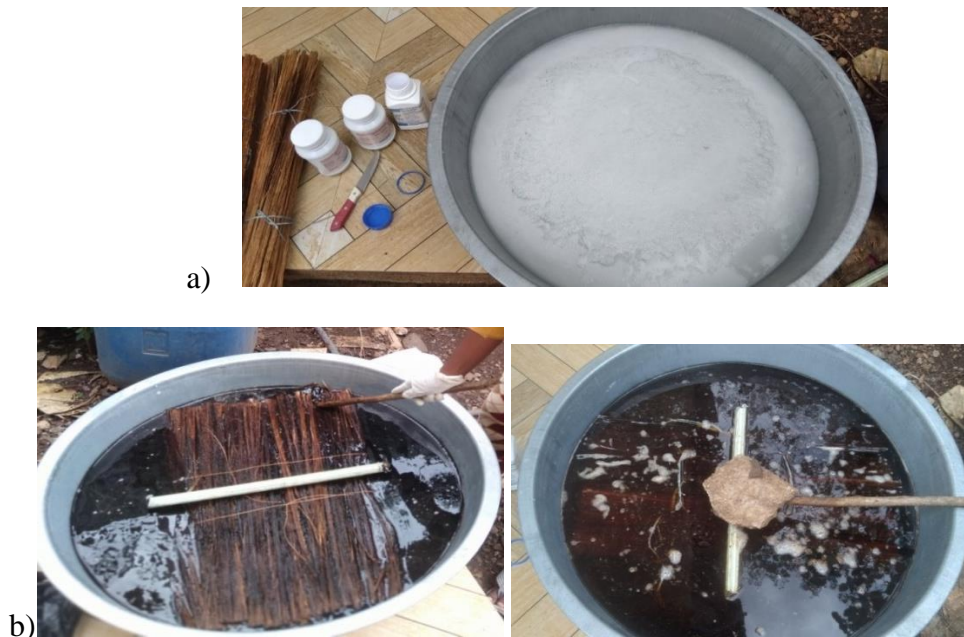
Figure 3-8 a) Alkali (NaOH) solution b) soaked bamboo fiber to extract lignin & hemicelluloses
