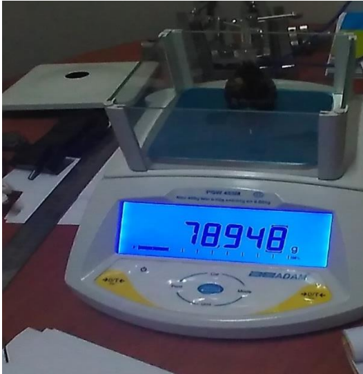
Figure 3-9 density measurement of bamboo fiber using picnometer
