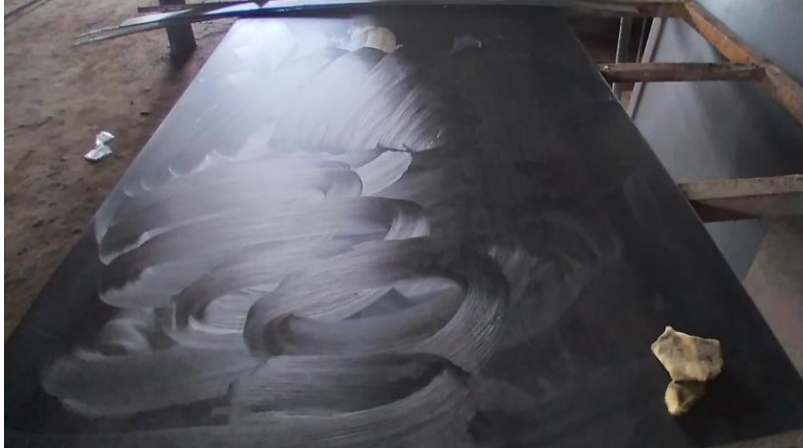
Figure 3-10 sheet metal mold cleaning and polishing mold with releasing agent (wax) for easily releasing of the composite plate after curing and for better surface finishing
