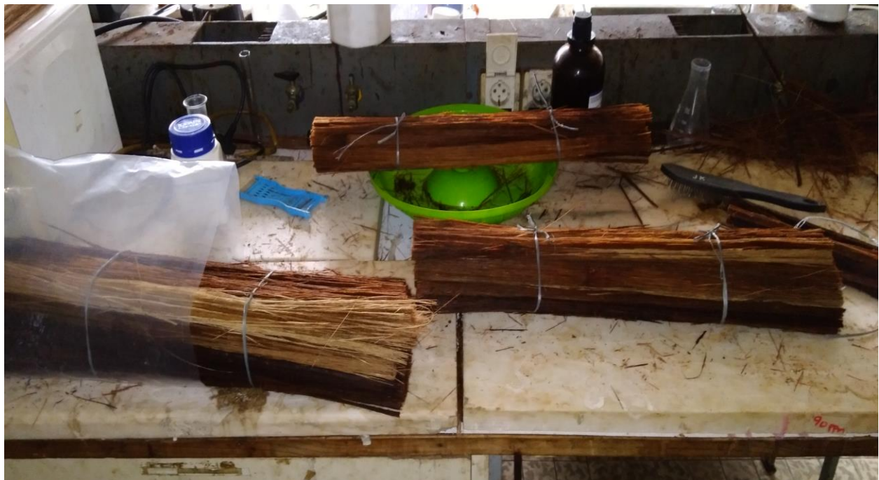
Figure 3-6 bamboo fiber soaked in tap water for 48 hours to soften it for further mechanical extraction
