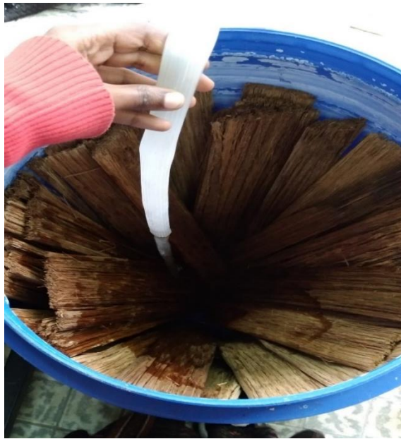
Figure 3-6 bamboo fiber soaked in tap water for 48 hours to soften it for further mechanical extraction
