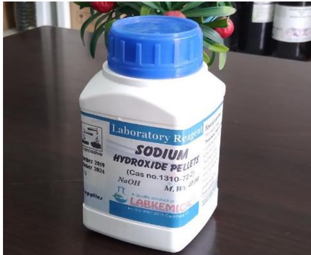
Figure 3-3 The Alkali (NaOH) used to treat the fiber order to extract lignin and hemicelluloses
