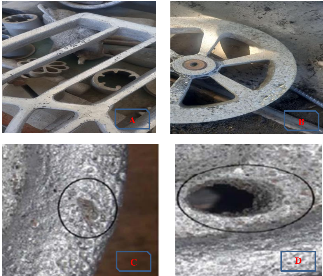
Figure 1.1:-Rejected pulley product due to defect (Photos taken from the case company)
