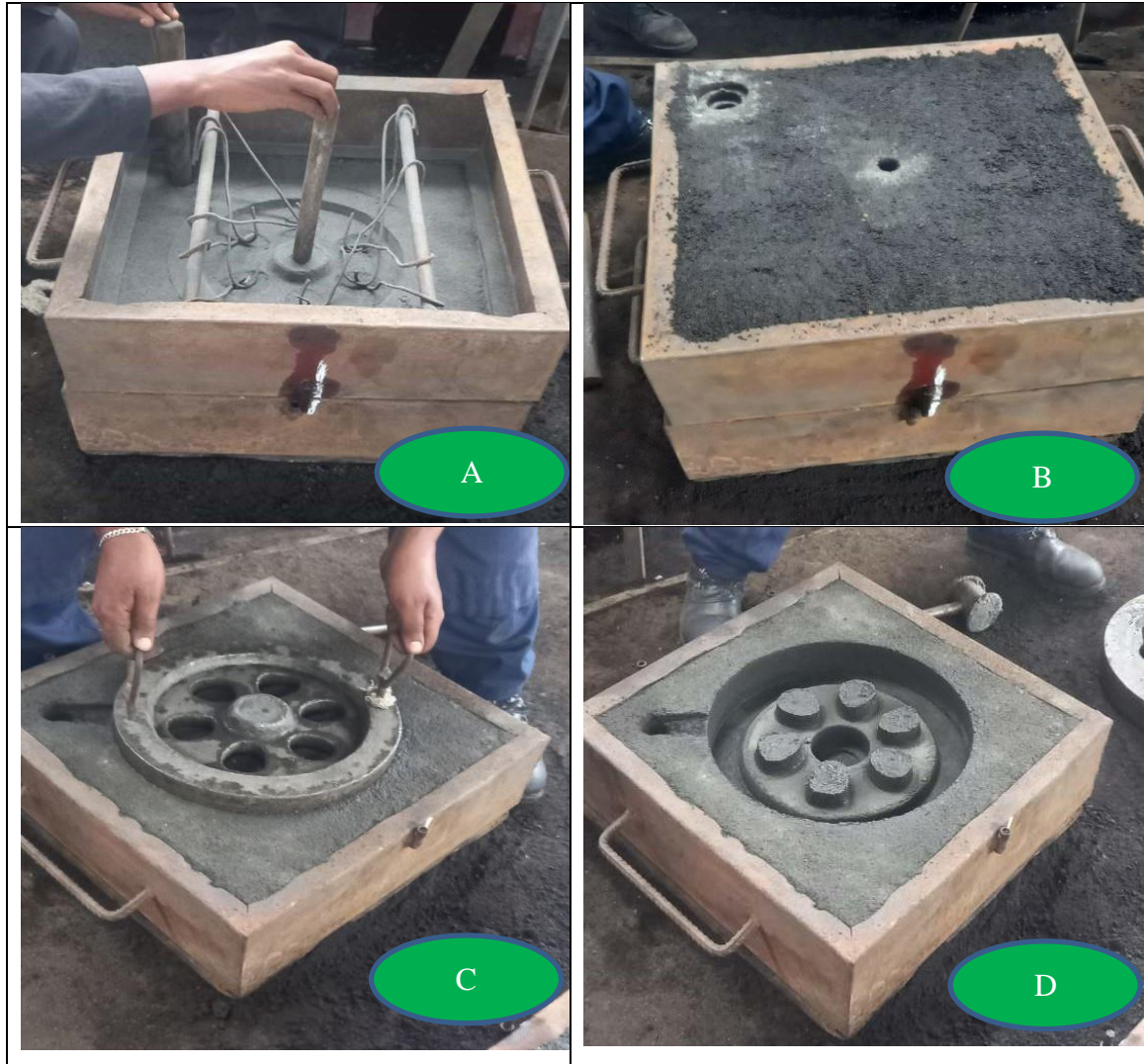
Figure 3.5:- Mold making process [Photo taken during experimental task at case company]
