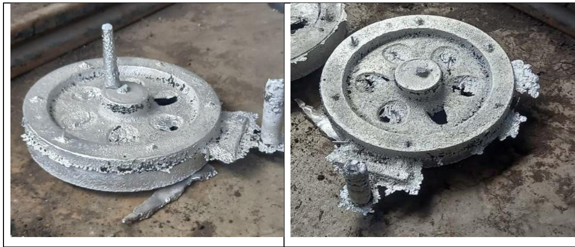
Figure 3.15:- Fabricated pulley product according to selected simulation result (Trial Order seven)
