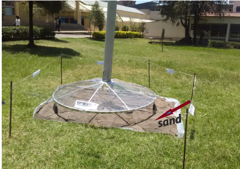
Figure 4-19: sand placed beneath the collector
