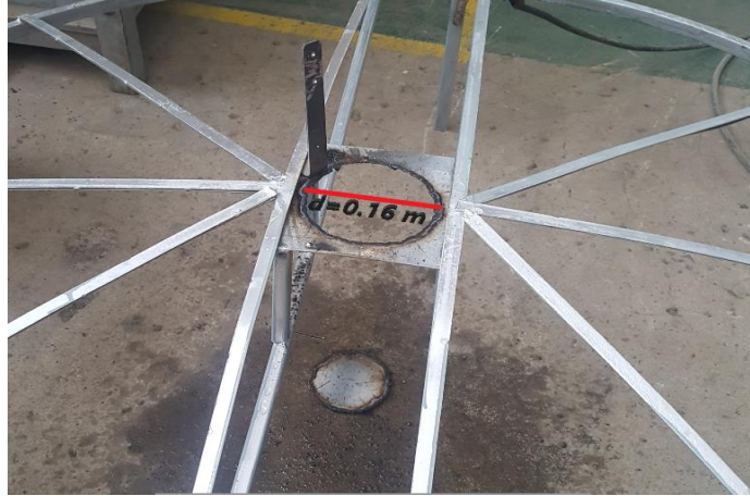
Figure 4-13: Hole preparation as a collector exit
