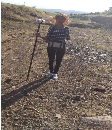
Figure4.2 Magnetic data acquisition in the study area
