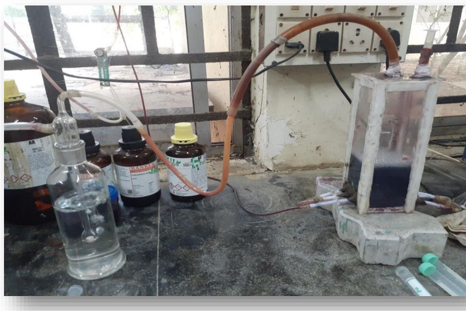
Fig.1 Apparatus for VOC stripping and condensation
