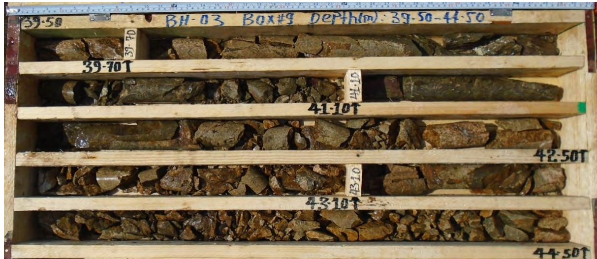
Plate 6.1 Rock core showing zone of weakness, decomposition at the contact zone (Borehole 3)
