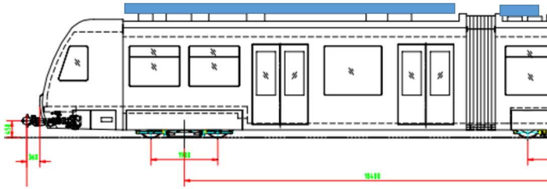
Figure 3-2: Section of the train showing where the solar panels (in blue) shall be installed
