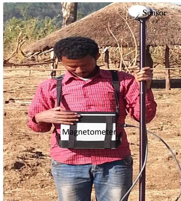
Figure4.13. Magnetic data acquisition using the GSM-19T magnetometer.
