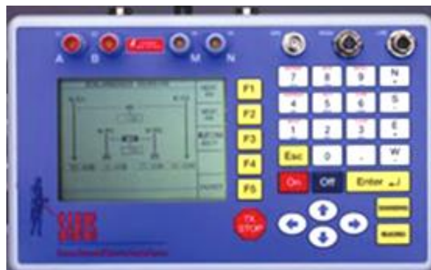
Figure 4.5. Front panel of the SARIS Terrameter.
