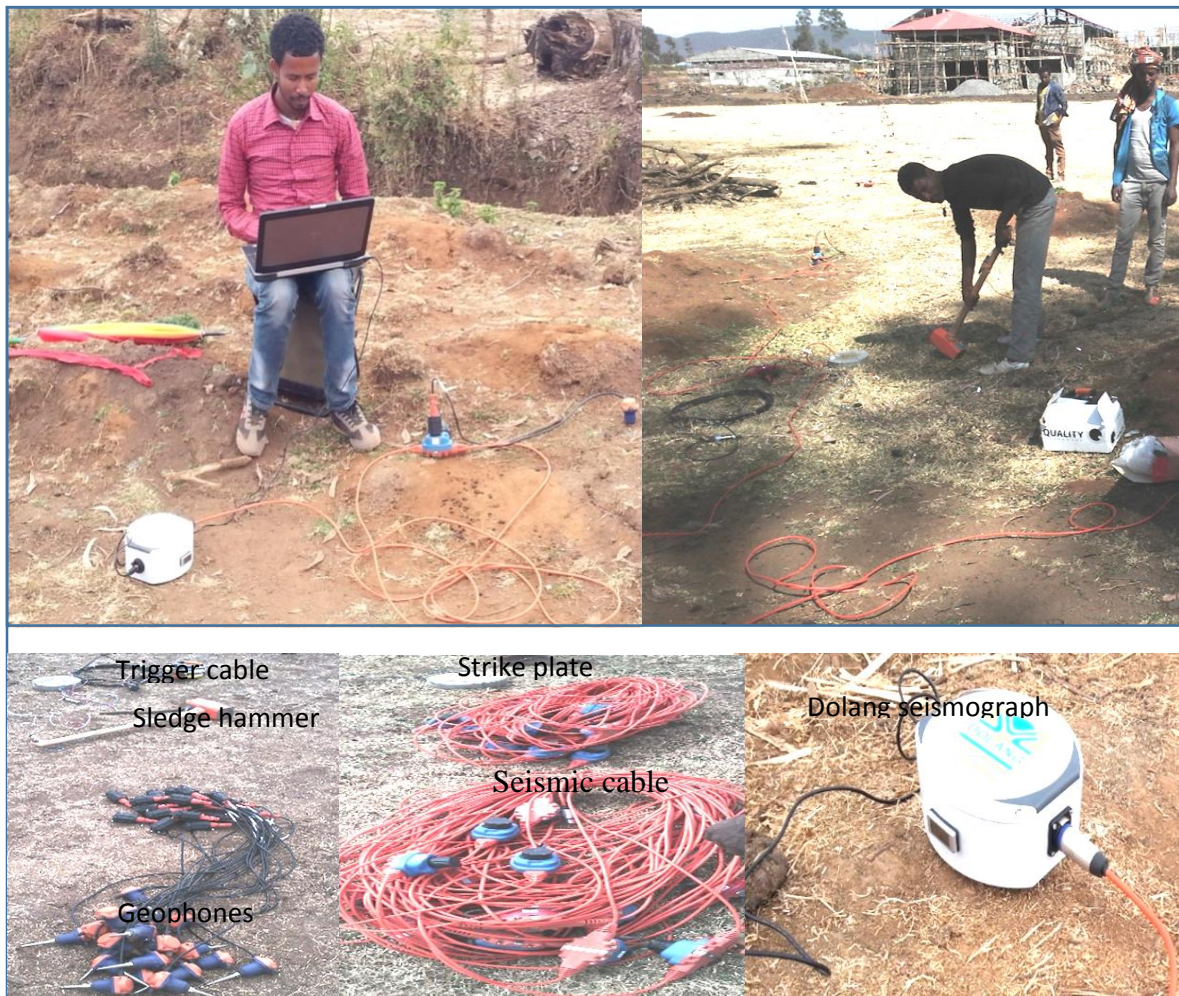
Figure 4.9. Field setup, data acquisition and instrumentation of seismic refraction survey.
