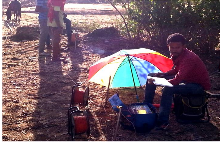
Figure 4.2. Field setup of the Vertical Electrical Sounding data acquisition
