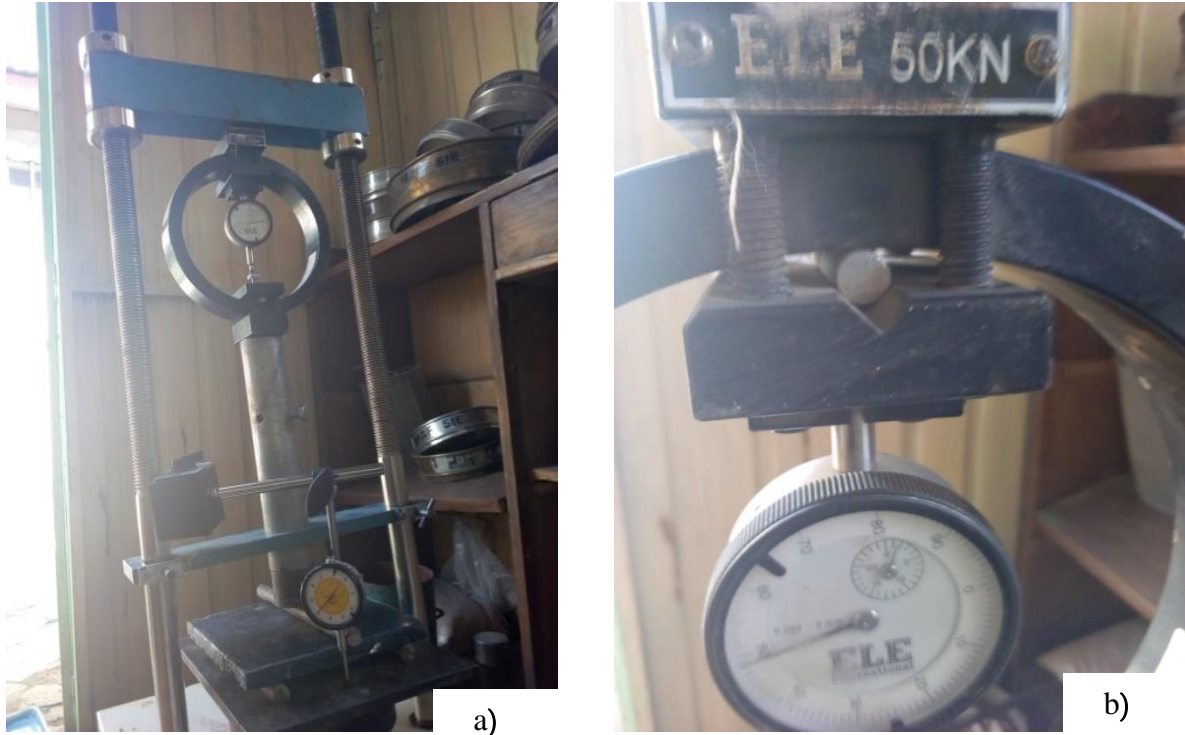
Figure 11: Setup of flexural strength testing machine
