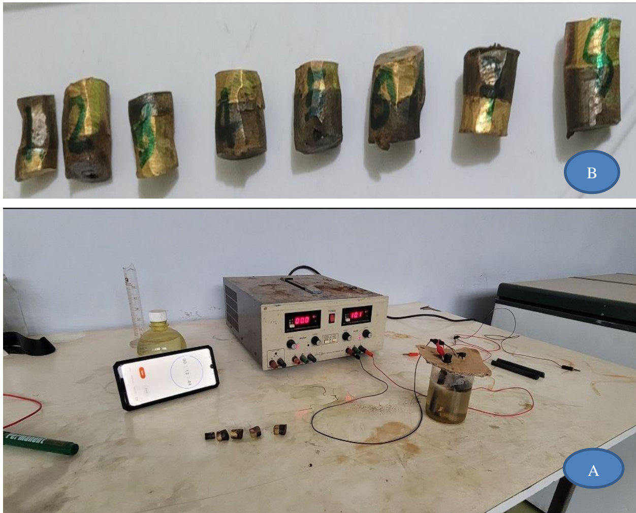
Figure 3.13 Electro chemical corrosion testing set up (A) and Sample prepared for corrosion test (B)
