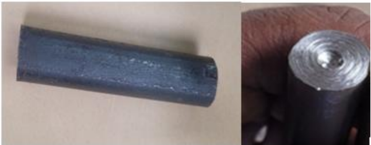
Figure 3.3 low Carbon steel rod with dia 12mm and 15 mm
