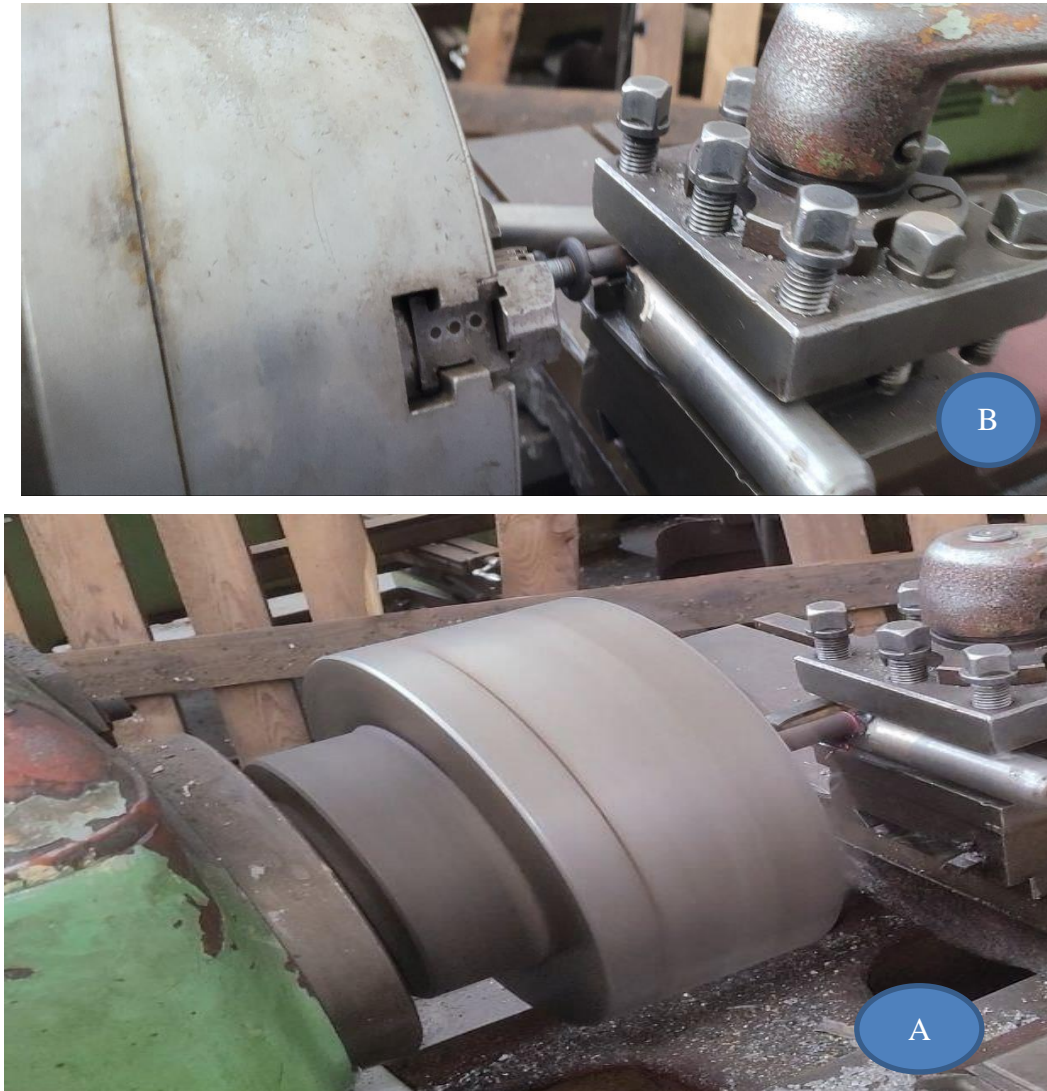
Figure 3.14 Lathe machine specimen clamp (A) and lathe machine vice (B) (Photo taken from from AAU AAiT mechanical work shop)
