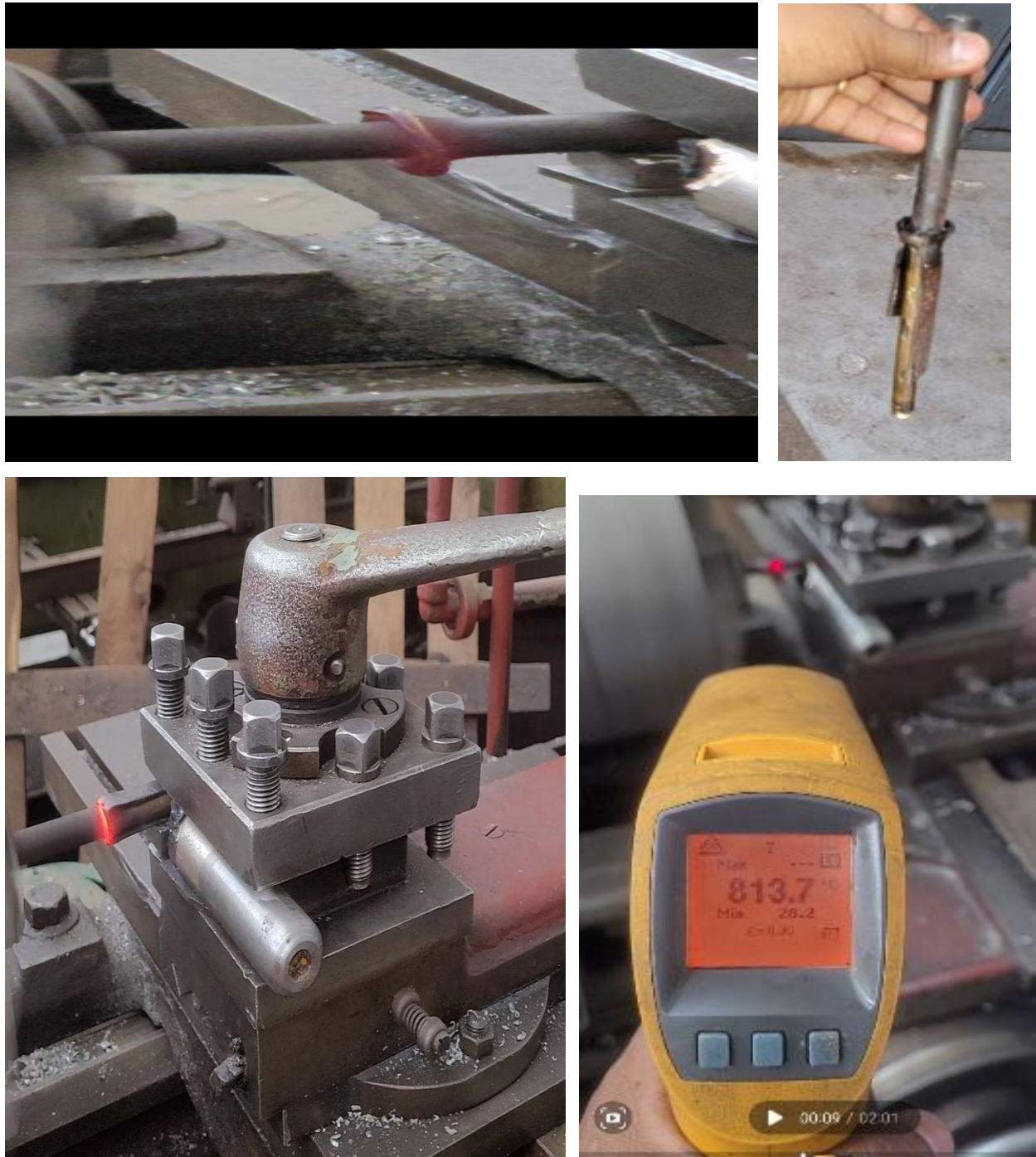
Figure 3.15 Welding experimental process records on lathe machine
