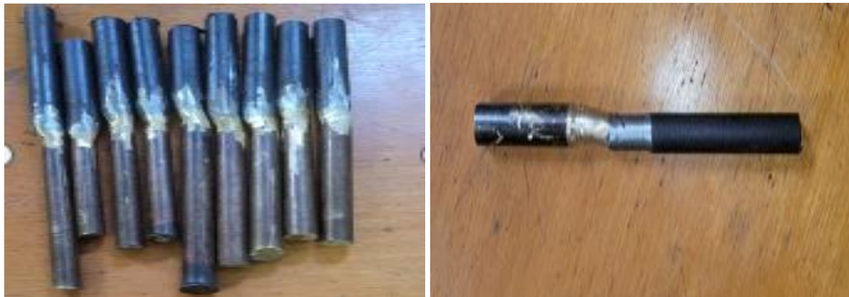
Figure3.11 Welded part before extraction of tensile specimen
