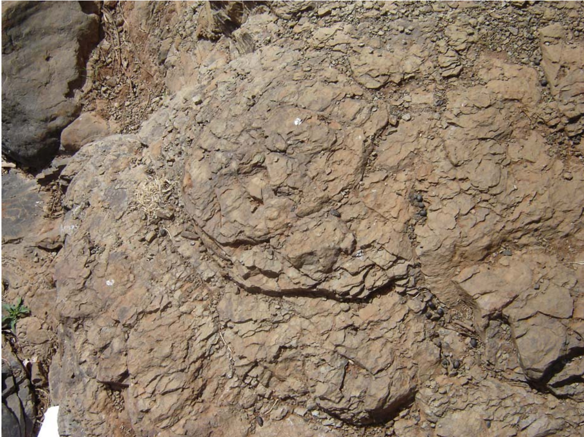
Figure 5.7 weatherd and fractured Alaji basalt (Adopted from Ketema Wogari, 2006)
