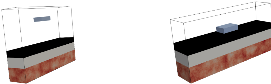
Figure 3.6: Typical Asphalt Pavement Simulated on gprMax with Air Suspended and Ground coupled antennae
