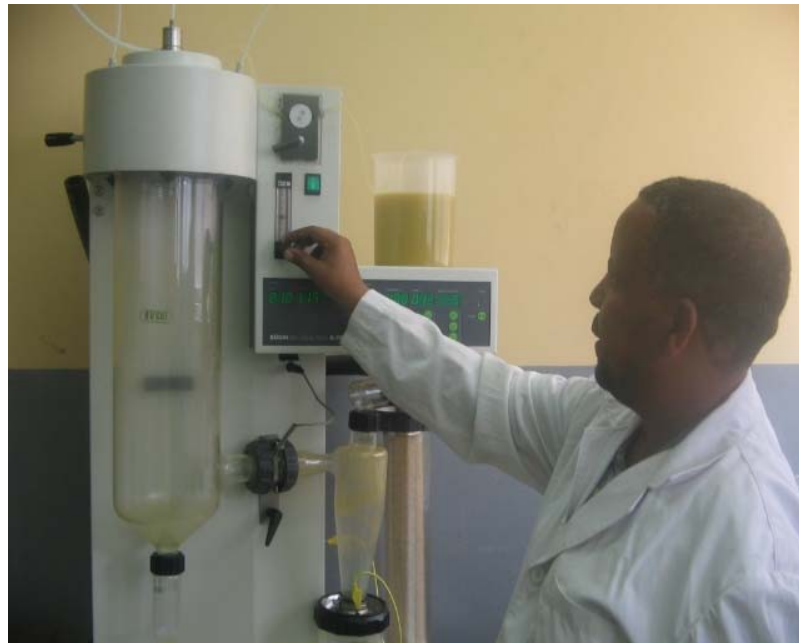
Fig3.4. Spray drying process
