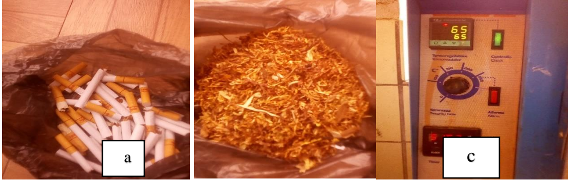
Figure 3.3 Moisture content determination a) cigarette butt; b) tobacco filler; c) Drying of tobacco filler under oven
