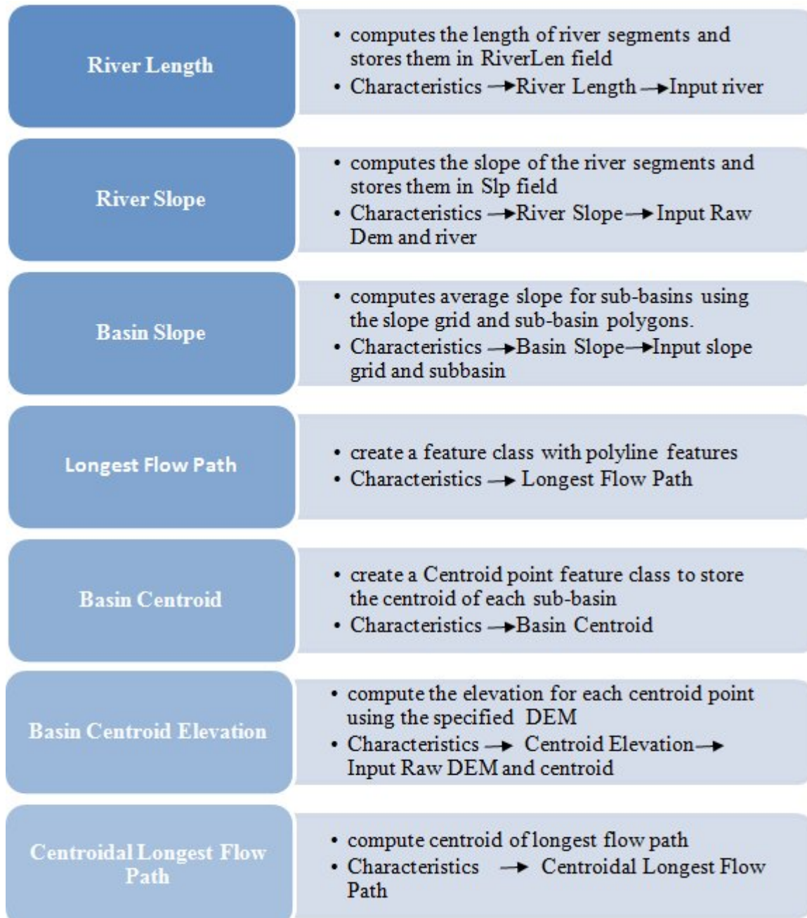
Figure 3-4: Process of extracting physical characteristics of sub basin and rivers Some of these physical characteristics are stored in attribute table of the features where others like centroid and longest flow path are displayed with the help of points and polyline respectively.
