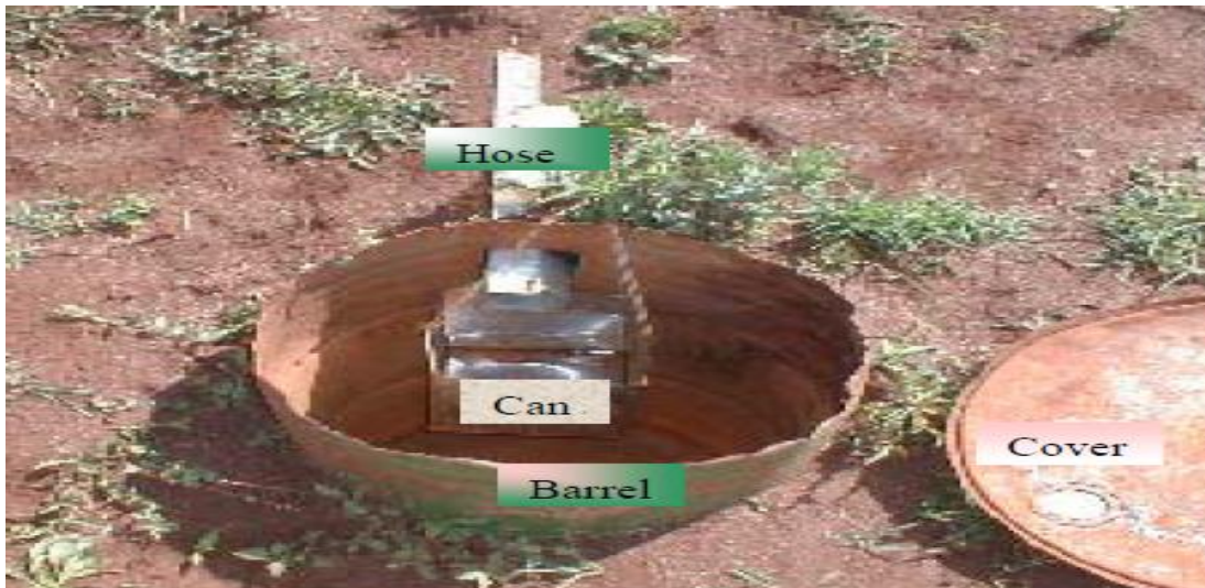
B. Runoff collectors
