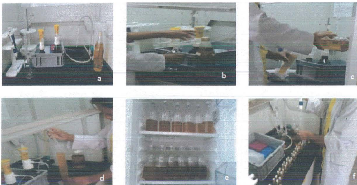
Figure 3.2: Sample preparation (a) internal standard working solution in a tray with melting ice. (b) 2.0 ml of the cold internal standard working solution added into an infusion bottle, (c), beer sample were slowly filled in a 250 ml graduated measuring cylinder. (d) The excess of beer and/or foam were removed by using a water jet suction pump to obtain 250 ml. (e), each infusion bottle was kept in refrigerator (f) Auto sampler vials filled with the prepared samples.
