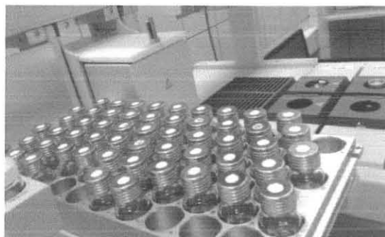
Figure 3.3. Beer samples in auto sampler vials on auto sampler tray
