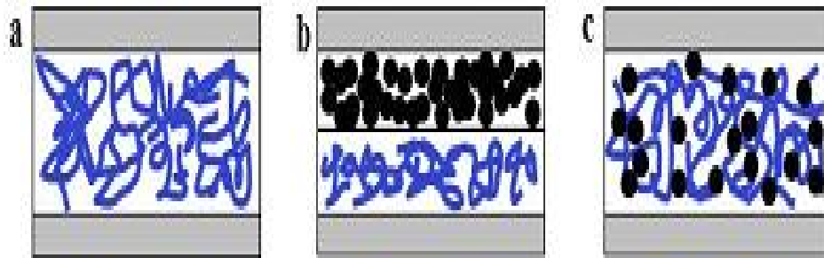
Figure 2.9: Schematic comparison of solar cell architectures; (a) single layer (b) bilayer and (c) BHJ with polymer- (blue) and PCBM-rich (black) phases.
