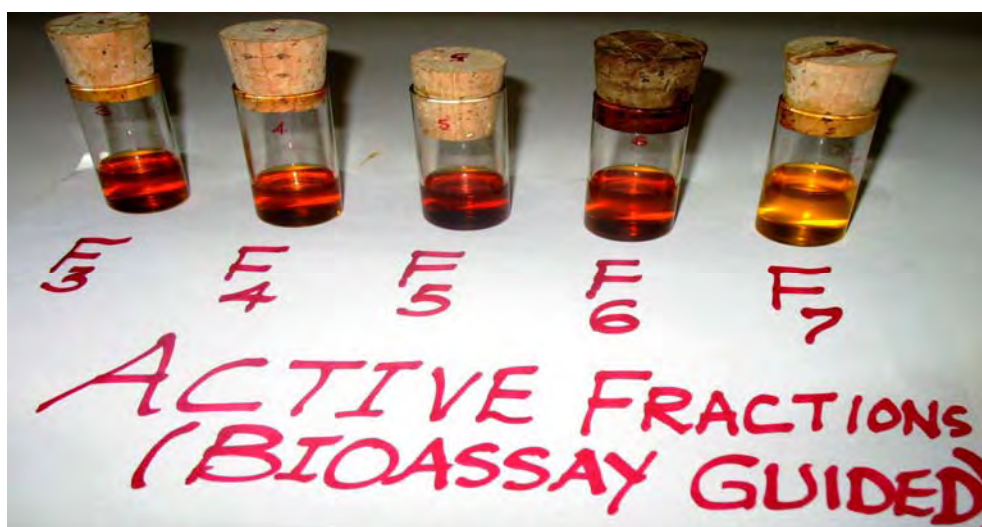
Fig.13 Active fractions collected from column chromatography
