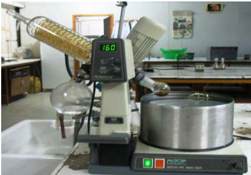
Fig.4 Extraction method: Rota-vapor set at 160 rpm and 60°C
