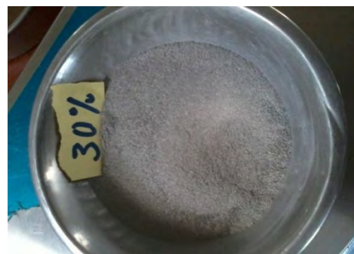
Fig. 5.9 30% marble dust blended sample prepared for Atterberg limit tests
