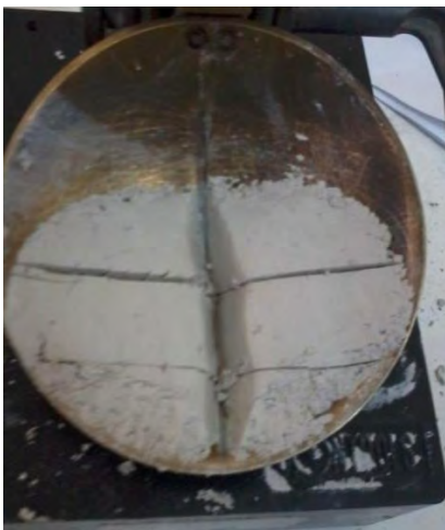
Fig. 5.7 Atterberg Limit test on the marble dust
