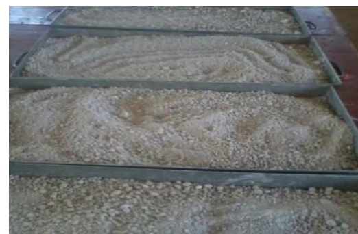
Fig.5.10 Marble dust blended sample prepared for Proctor and CBR tests
