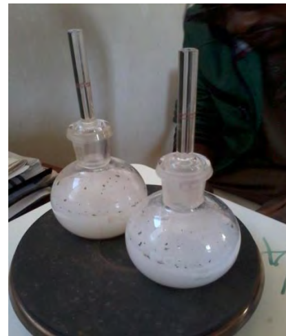
Fig. 5.8 Specific gravity test for marble dust
