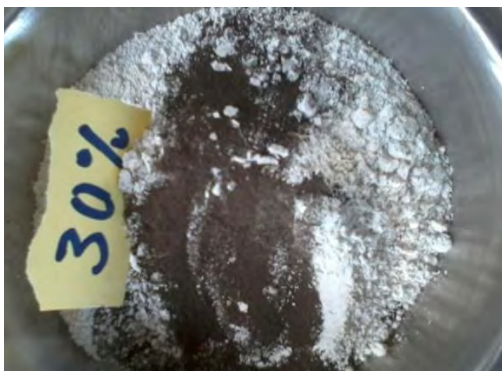
Fig. 5.9 30% marble dust blended sample prepared for Atterberg limit tests
