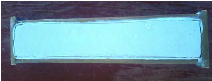
Fig. 5.6 Shrinkage test for marble dust (after oven drying)
