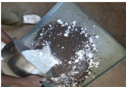
Fig.5.10 Marble dust blended sample prepared for Proctor and CBR tests
