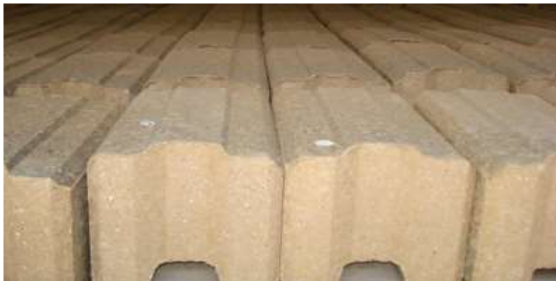
Figure 2-4: Interlocking CSSB at Selam Technical and Vocational Center, Addis Ababa.
