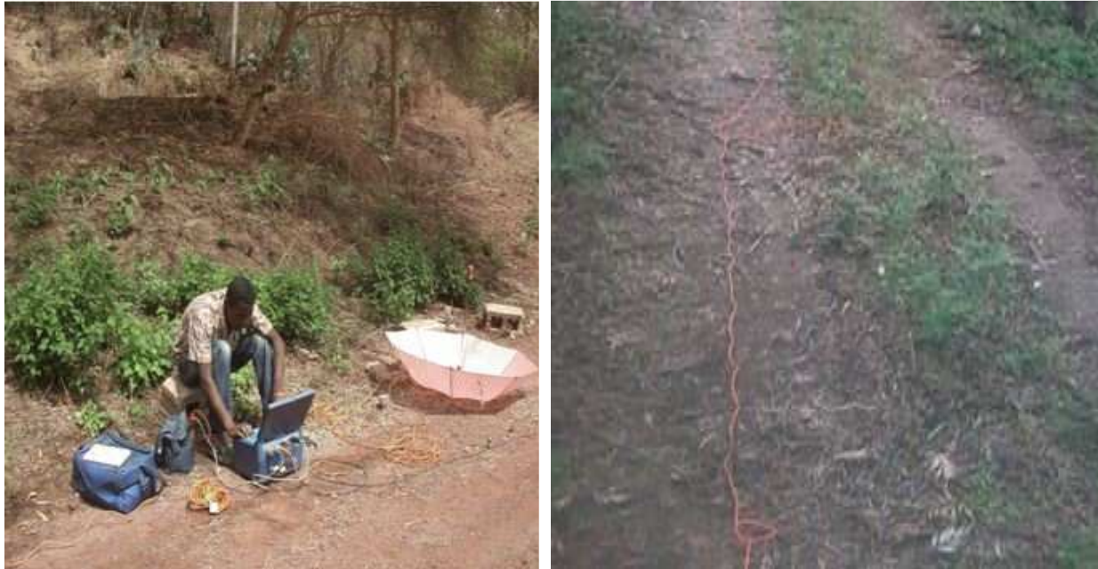
Figure 9. Field setup of seismic survey photo.
