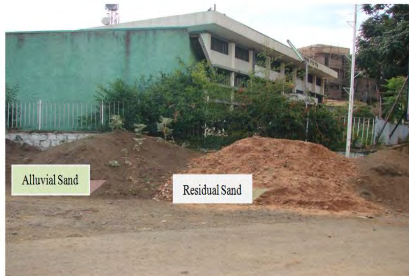
Plate - 6.8 Residual and Alluvial Sand/ Sand-gravel Mixtures for Local Constructions (in Debre Markos City)
