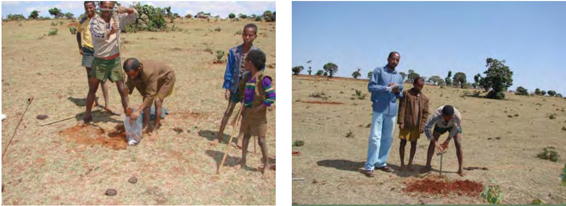
Plate - 6.7 Impermeable Soil Borrow Area1; Sampling and Auguring/ Logging
