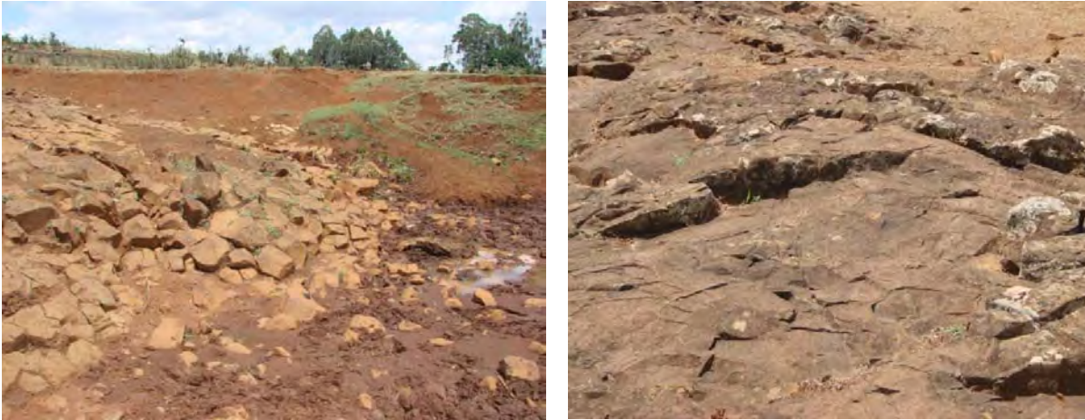
Plate 6.2 Top Jointed and Underlying Massive Foundation Basalt Rock (at right valley floor)
