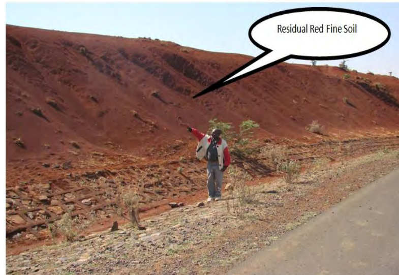
Plate- 6.6 Road Cut Exposure of Fine Grained Residual Soil in the surroundings of the Research Area
