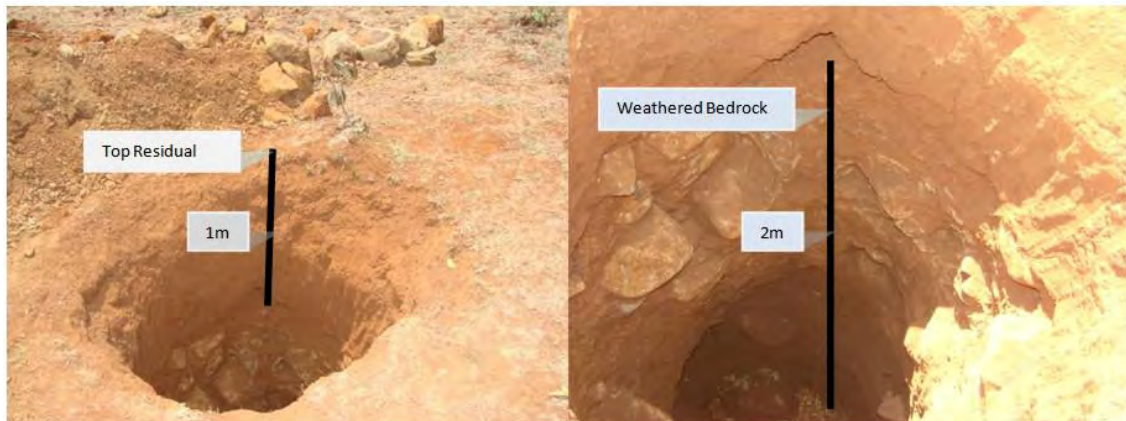
Plate - 6.4 Soil / Rock Profile at Right Abutment Foundation Area (from pit SHFOTP-2)
