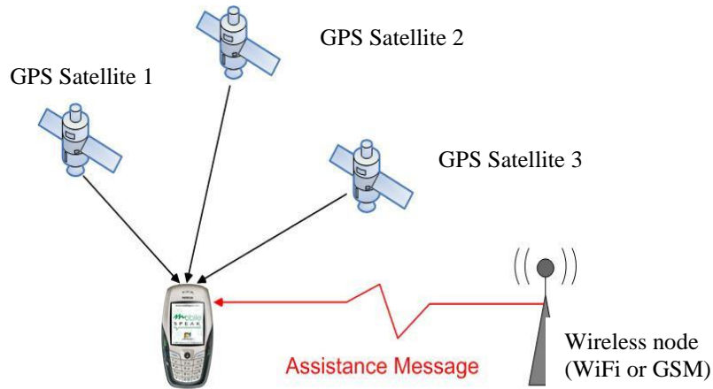
Figure 2-2: Principle of A-GPS
