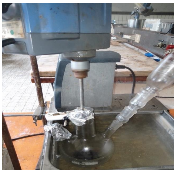
Figure 0-9 Experimental setup for transesterification reaction
