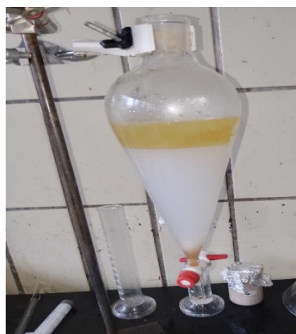
Figure 0-11 Degumming of ethyl ester
