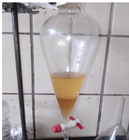
Figure 0-10 phase separation between ethyl ester and glycerol
