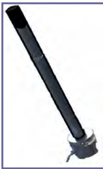
Figure 4.2: Collimator tube mounted on photodiode used as a detector for our pyrheliometer. The inside of this tube is blackened to block circumsolar sky radiation.
