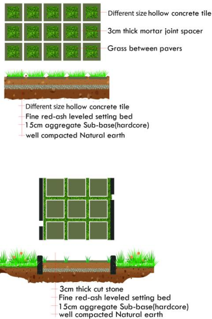
Figure 4-19: Pervious Pavement detail(Author, 2020)
