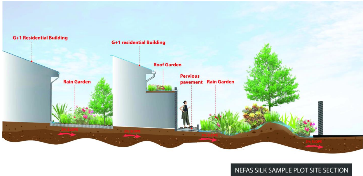
Figure 4-14: Lebu Varnero apartments 500m 2 sample plot GI measures cross-section plan (Author, 2020)
