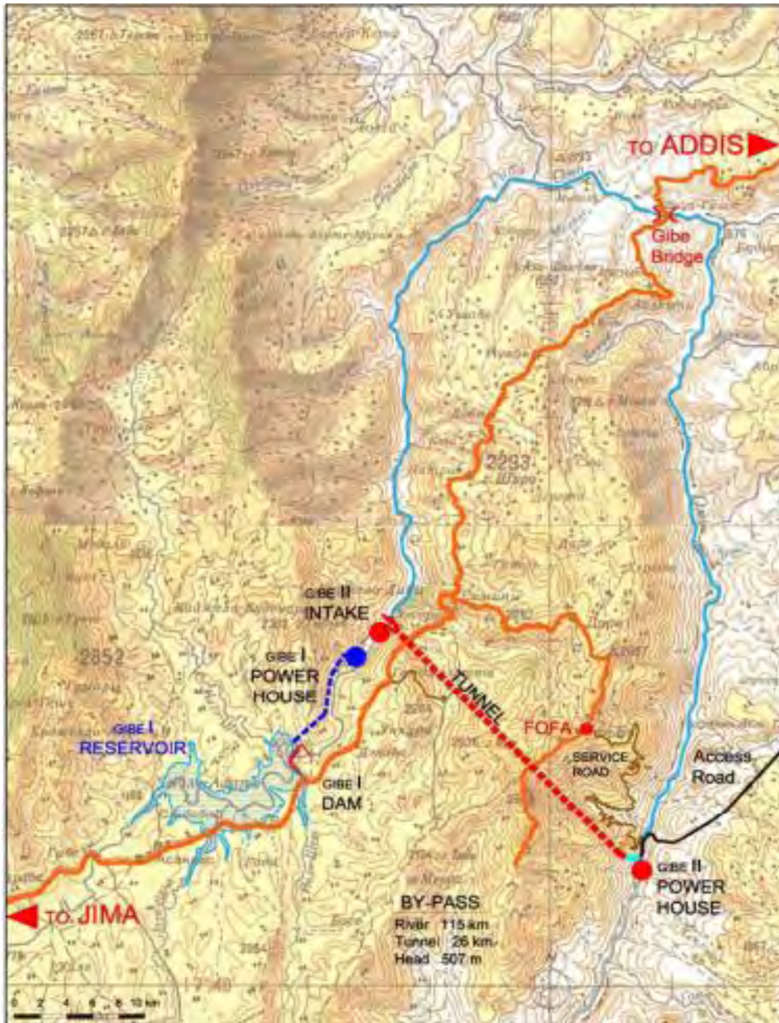
Figure H.1 General Layout of the Gilgel gibe-I and II hydroelectric system.
