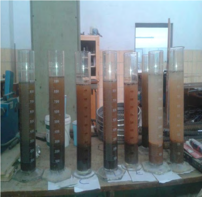
C.5 Photo: Silt content test Photo:
