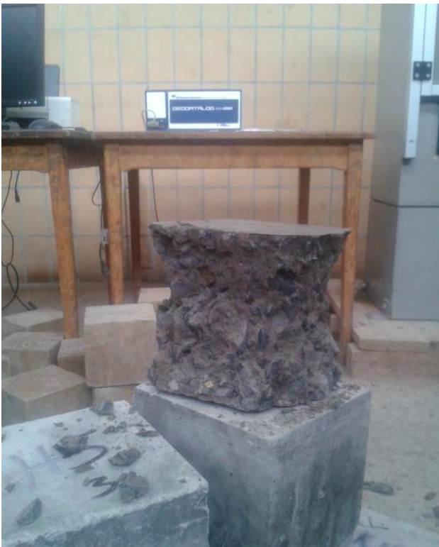
C.3 Photo: Failure Mode of river sand
