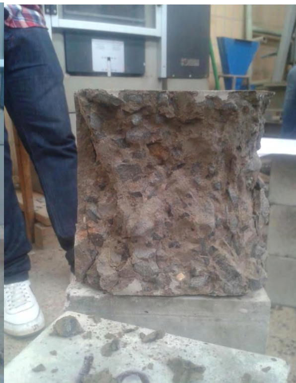
C.4 Photo: Failure Mode of Jema sand
