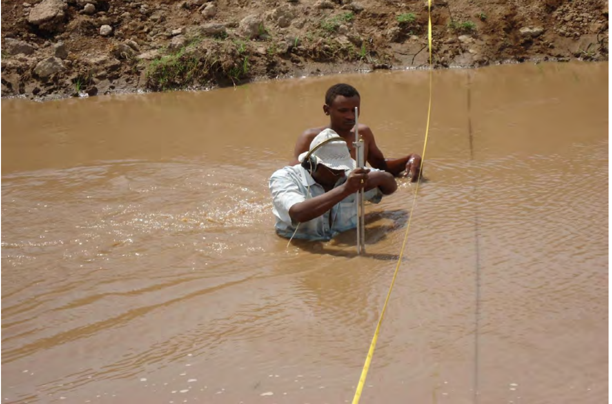
Figure 3.3 Main canal discharge measurement at Fantale irrigation project
