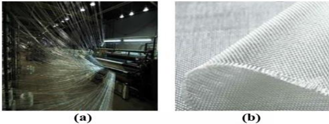
Figure 5: Digital images of a) unwound glass fibers, b) woven glass fibers [13]
