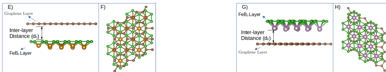
Figure 14: The optimized structures of MBene Based hetero-structures. (E) side view of graphene/B_2Fe . F) Top view of graphene/B_2Fe . G) side view of B_2Mo/graphene . H) Top view of B_2Mo/graphene .
