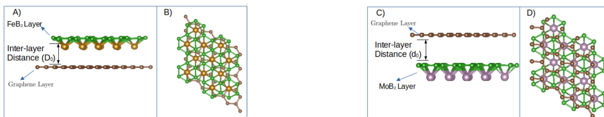
Figure 13: The optimized structures of MBene Based hetero-structures. A) side view of B_2Fe/graphene . B) Top view of B_2Fe/graphene . C) side view of graphene/B_2Mo . D) Top view of graphene/B_2Mo .
