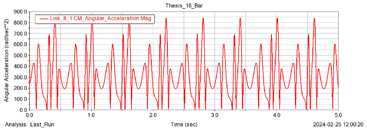
Figure – B.34: Angular Acceleration versus Time of Link_8_1 for Five Seconds of Simulation
