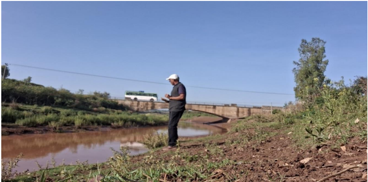
Plate 1. Measuring the width and depth of the Awash River downstream of the main bridge.
