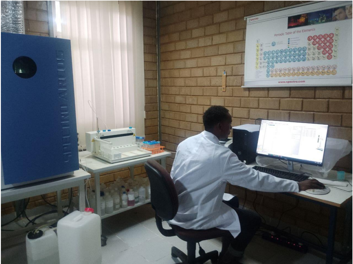
Analysis of Aqueous Solutions by ICP-OES with radial plasma Observation
