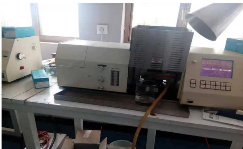
Figure 4.11 Detection of Arsenic content by Atomic Absorption Spectroscopy
