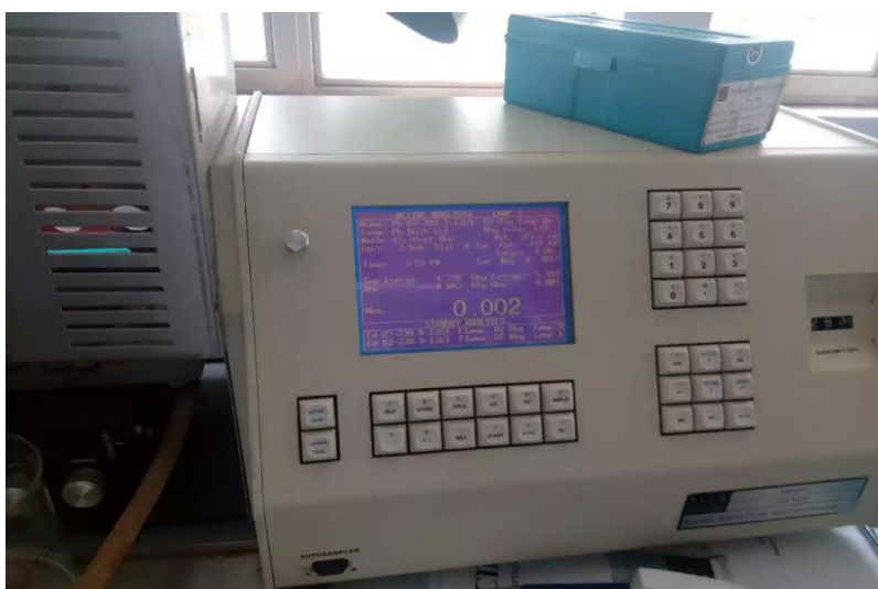
Figure 4.10 Detection of Iron content by Atomic Absorption Spectroscopy
