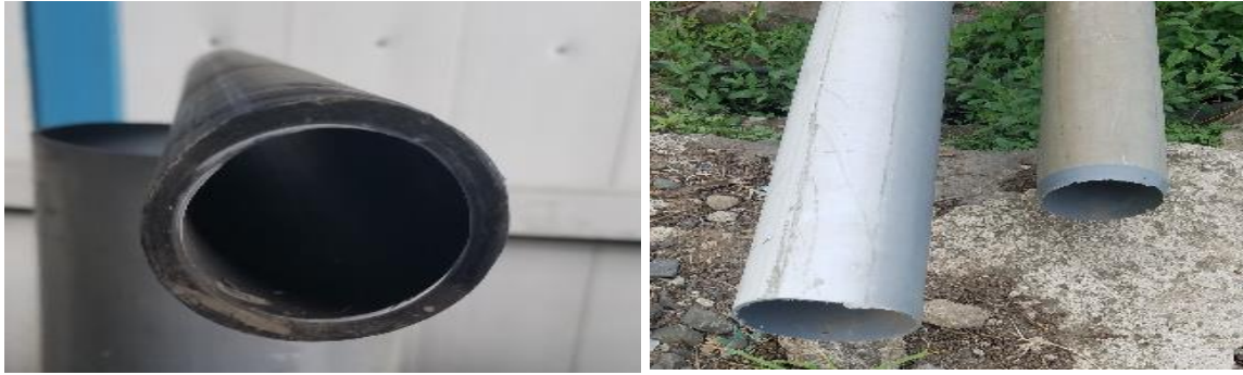
Figure 14: Observed quality defect thickness variation and width variation
