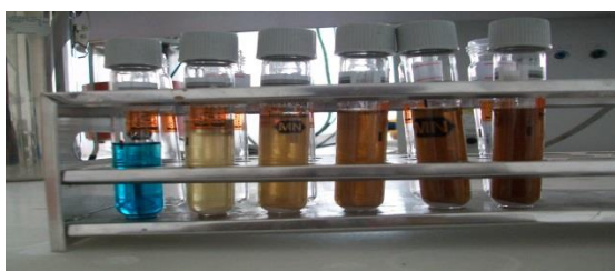
Figure 4.1 Standard glucose solutions after being reacted with benedict's solution (reagent)
