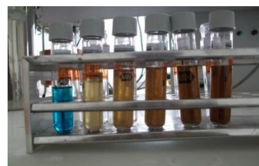
Std. glucose solution after being reacted with Benedict's reagent
