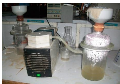
Vacuum filtration machine
