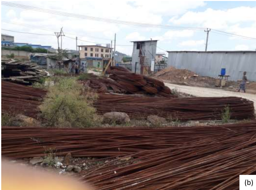
Figure 4.8: Unused Rebar that corrodes due to excess stock
