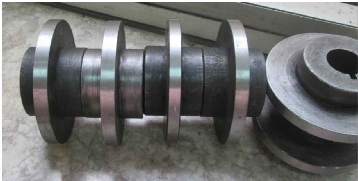
Figure 3. 12: photograph of wheel and rail contact surface before test
