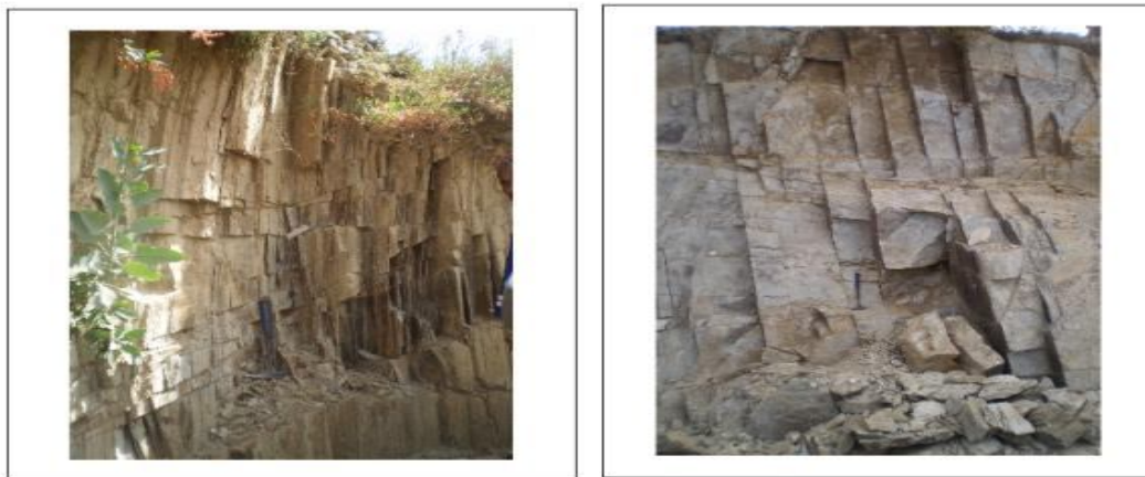
Fig 19 Sub-horizontal and sub-vertical closely spaced systematic joint sets in the slaty rocks (561952 E, 1537751 N) (a) and phylitic rocks (564388 E, 1537965 N) (b) around Negash.
