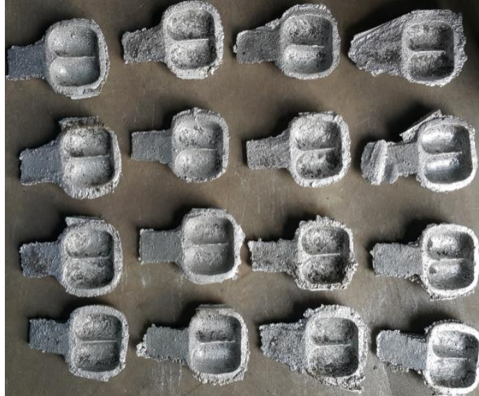
Figure 3.6: Photography of casted buckets before machining
