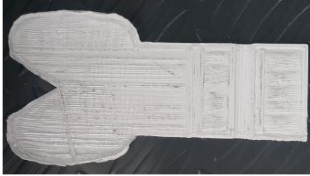
Figure 3.3: Photography of failed 3D printed optimized Pelton bucket in icogLab's 3D Printer
