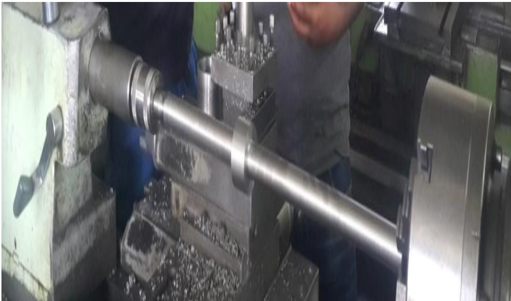
Figure 3.14: Photography of Turbine Shaft
