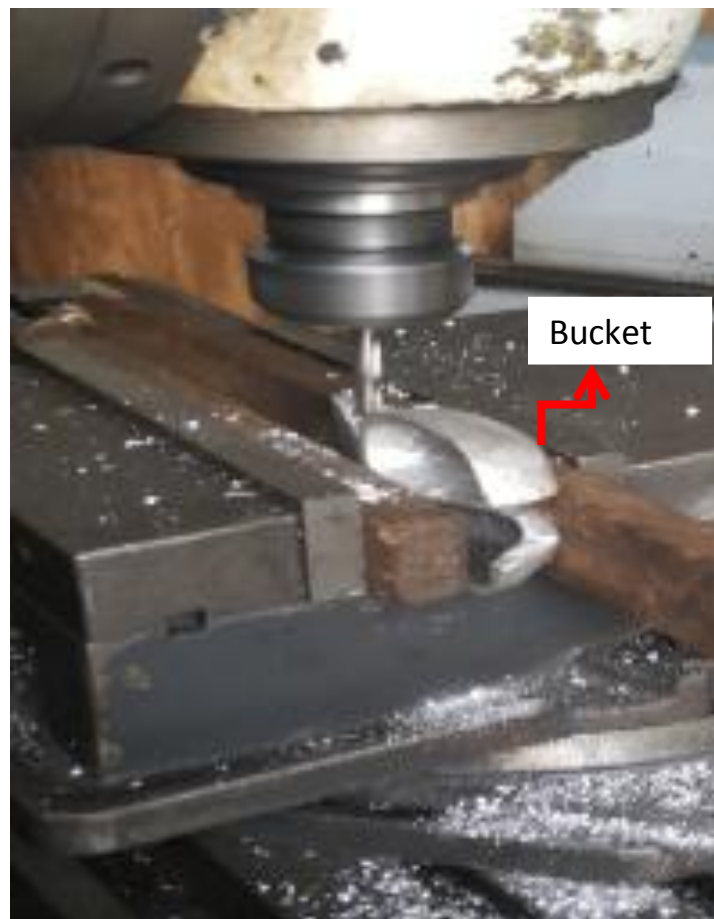
Figure 3.8: Photography of drilling of casted buckets
