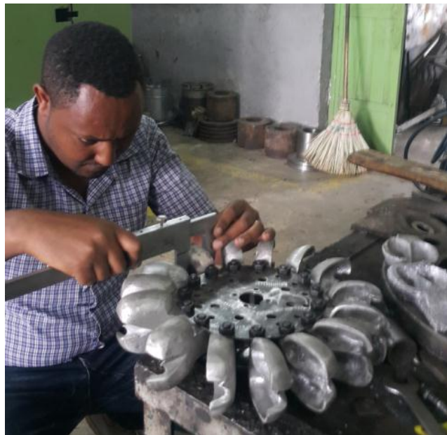
Figure 3.20: Photography of fixing of bucket with M8 Bolt to set the distance between each bucket
