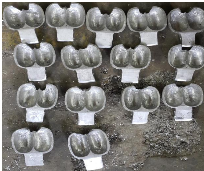
Figure 3.7: Photography of casted Buckets after machining
