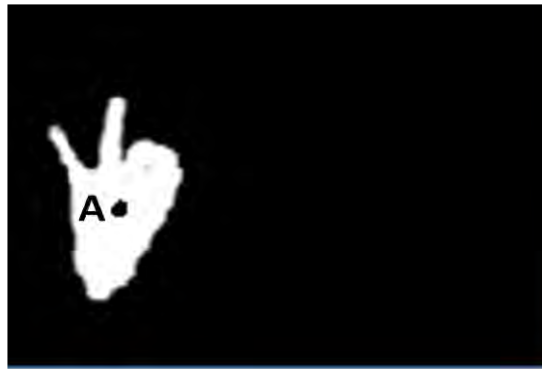
Figure 4.8 An image showing a centroid of an isolated hand
