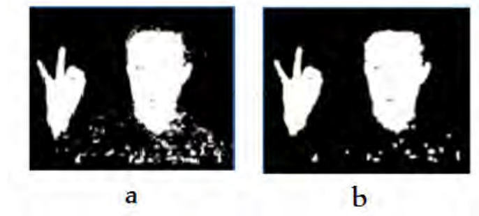
Figure 3.5 Morphological operations: a) Before opening and closing b) After opening and closing
