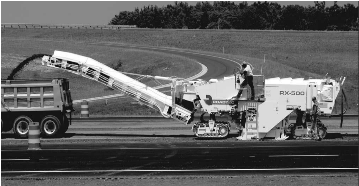
Figure 2. Typical Front-Loading Milling Machine
