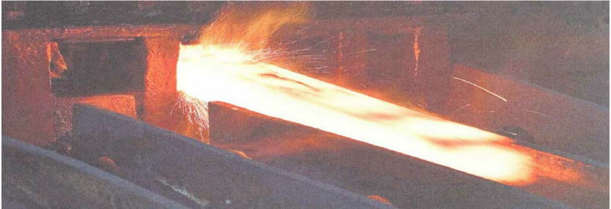
Figure1.7 Rough pass in a hot rolling mill [ 8]
