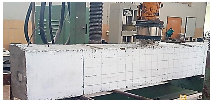
Figure 4-1 beam test setup
