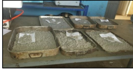
Figure 5.7: Soil treated with cement and molasses (front) and soils treated with cement (back) after curing period
