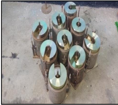
Figure 4.8: Curing CBR test specimen at room temperature (left) and wet drying (right).
