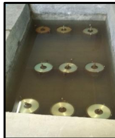
Figure 4.9: Measuring swell value at the beginning & end of soaking (left) and Soaking CBR Test Specimen (Right)
