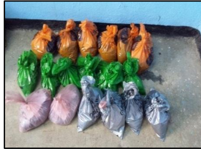
Figure 4.4: Specimens prepared for Atterberg's Limits (left) and curing (right)
