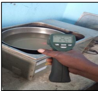
Figure 4.2: Preparing water bath at 25 \pm 1^\circ\text{C} (Left) and soaking specimen in the water bath for 1 hour (Right).
