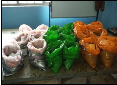
Figure 4.4: Specimens prepared for Atterberg's Limits (left) and curing (right)
