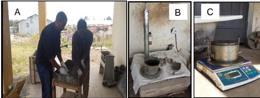
Figure 3.13: Proctor test. (a) Soil-water mixing, (b) apparatus for compaction test, and (c) weight measuring after compaction
