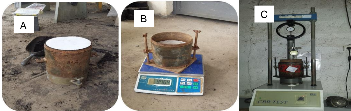
Figure 3.14: CBR Test Procedure: (a) & (b) CBR specimen preparation, and (c) CBR penetration.
