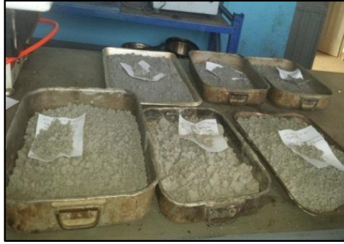
Figure 4.5: Oven dried specimen for Atterberg Limits after curing period
