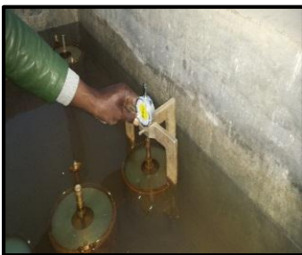
Figure 4.9: Measuring swell value at the beginning & end of soaking (left) and Soaking CBR Test Specimen (Right)
