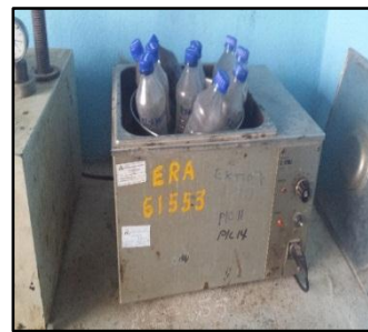
Figure 4.2: Preparing water bath at 25 \pm 1^\circ\text{C} (Left) and soaking specimen in the water bath for 1 hour (Right).
