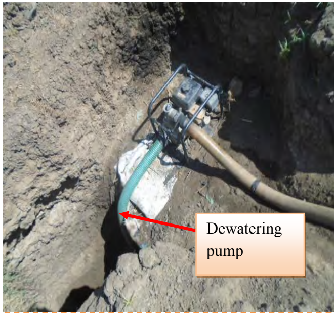
Plate 5.13 Hand dug well extraction for irrigation in Koka area (shallow Groundwater use trends)
