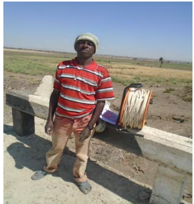
Plate 5.12 Dip meter which measures up to depth of 300m
