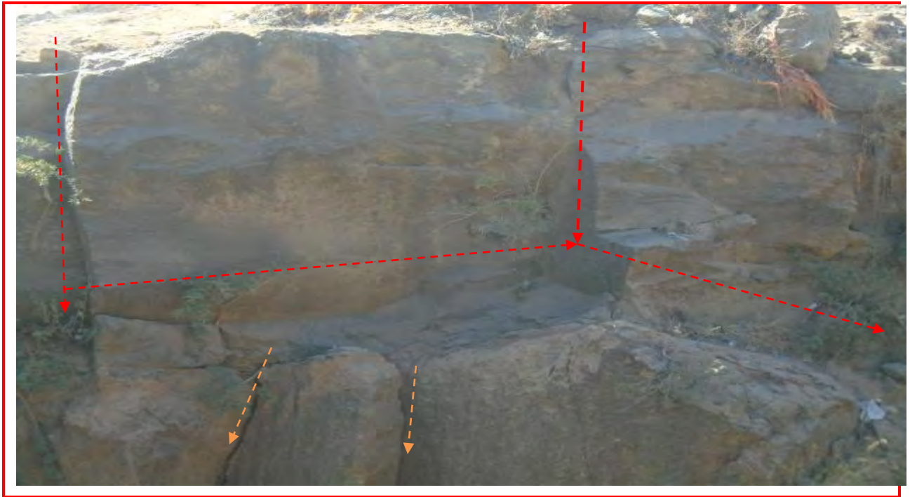
Plate 3.1 Columnar joint in ignimbrite rock unit in Mojo River side
